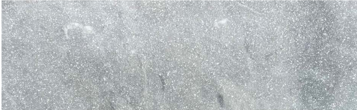
Plate 1: Appearance of Grey Marble with a sandblasted finish as received.
