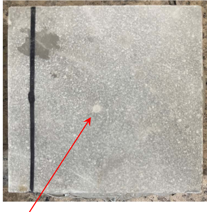
Plate 2: Appearance of stun mark on the surface of Grey Apricot caused by impact testing. Indent is approx. 3mm radius. (specimen M1285/22)
